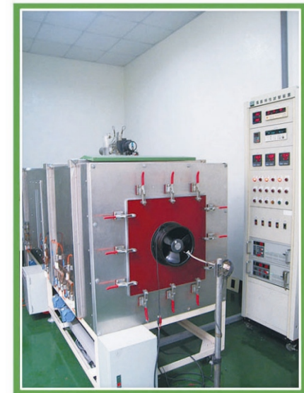
Air Flow Testing Machine
